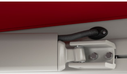
3 cable transition to the front profile
